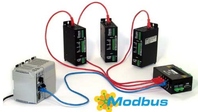
AMCI's [SD31045E](#) & [SD17060E](#) stepper indexer/drivers provide up to 4.5 Arms or 6.0 Arms (respectively) of output current and boast a wide range of features. In addition to Ethernet-based connectivity (Modbus-TCP & EtherNet/IP), AMCI's E-drives feature onboard indexers, encoder feedback, microstepping, programmable output current, anti-resonance circuitry, vari-step velocity control, compact design, and simplified set-up.
